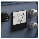
Each Kraftform Kompakt VDE set has been tested individually at 10,000 volts, in accordance with IEC 60900.This ten-times-higher testing load guarantees safe working at their maximum permitted load of 1,000 volts.
